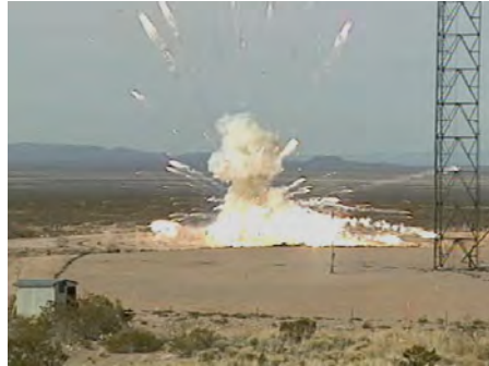
STAR 48 Destruct Test Using Model 2011 CSC
