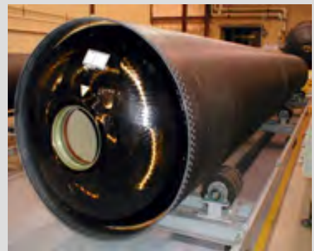
GEM cases are produced using advanced filament winding techniques developed and refined by Northrop Grumman for over 40 years
