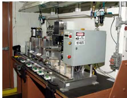
SCB Initiator Semi automated Manufacturing Line
