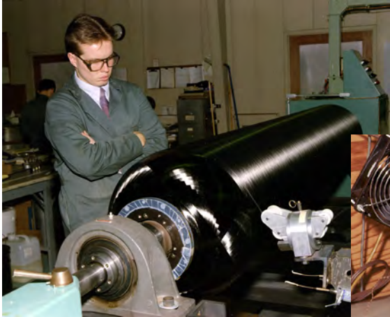
Graphite-Epoxy Composite Case Winding (21-in. booster)
