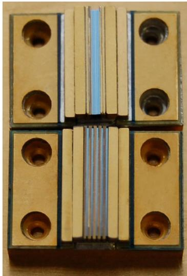
Northrop Grumman Cutting Edge Optronics has developed a new laser diode array package with minimal bar-to-bar spacing. These High Density Stack (HDS) packages allow for a power density increase on the order of  $\sim 2.5x$  when compared to industry-standard arrays.
