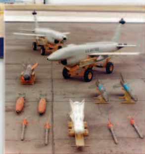
The First UCAV? BGM-34Bs demonstrated weapons delivery capabilities during the early 1970s in testing at Hill Air Force Base, Utah.
