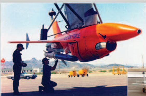
The First UCAV? BGM-34Bs demonstrated weapons delivery capabilities during the early 1970s in testing at Hill Air Force Base, Utah.
