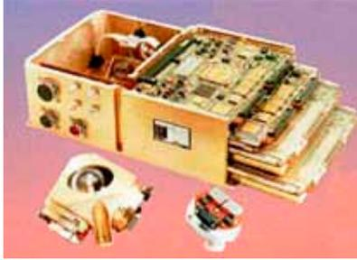
*Figure 15. HRG 130Y based Space Inertial Reference Unit (SIRU)*
