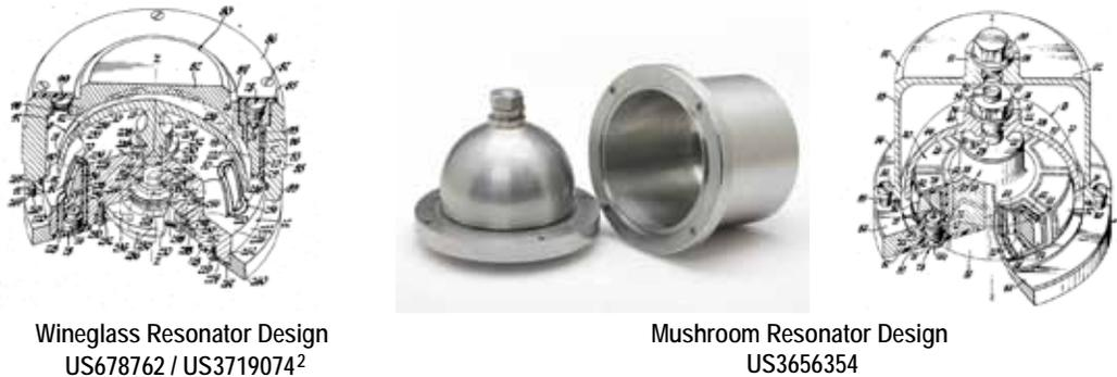
*Figure 4. Proof of Concept Designs – First HRG Gyros Built*
