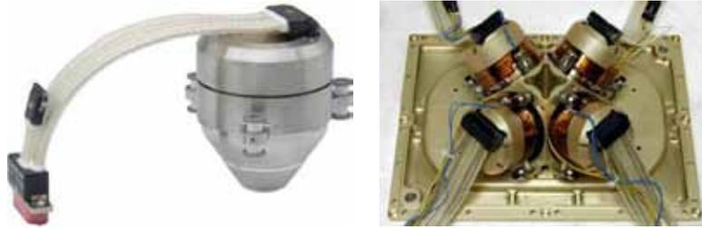
Figure 18. HRG 130P gyro and SSIRU Octahedral Tetrad Mount Platform
