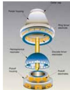
*Figure 13. HRG 158Y Production Gyro for Carousel-400 Aircraft Navigation System*
