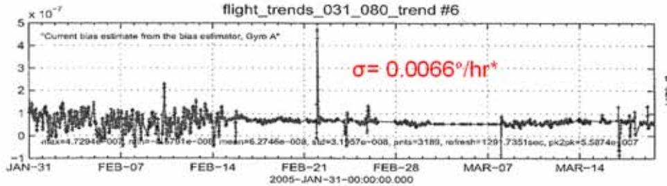
Figure 43. Deep Impact Gyro Rate Data
