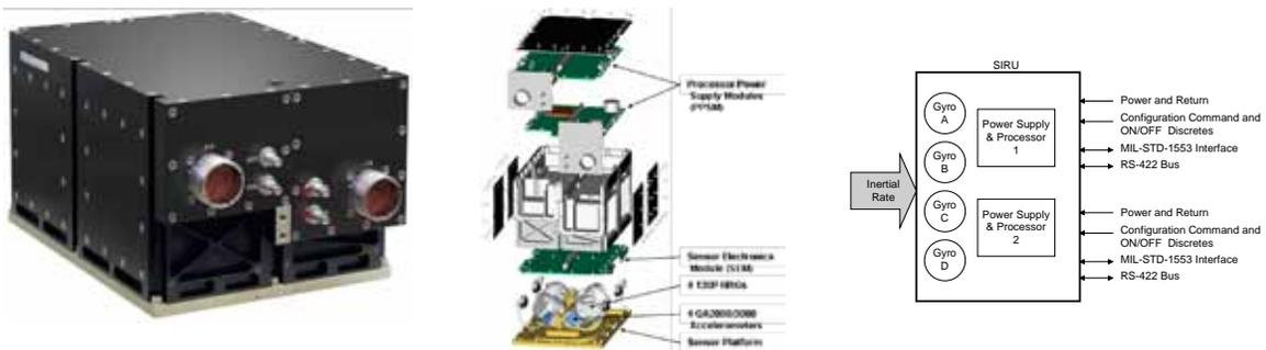
Figure 19. Scalable SIRU Unit, Exploded Assembly and Simplified Architecture Diagrams
