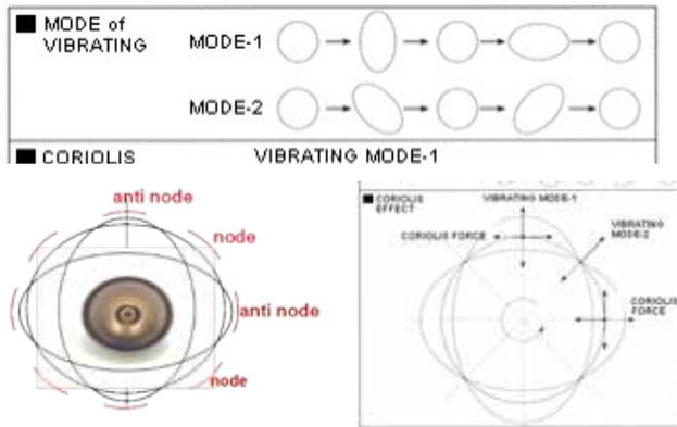
Figure 21. HRG Flex Motion in its Lowest Order Bending Mode
