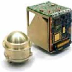
Figure 17. HRG for Hubble Rate Sensor Assembly
