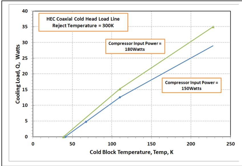
**Figure 3** – Performance of the coaxial HEC cooler at high cooling loads
