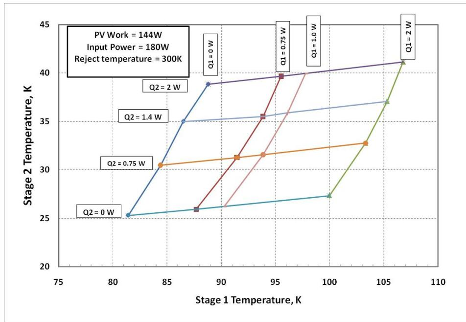
**Figure 6.** Performance map of the coaxial HEC Cooler at 300K reject temperature
