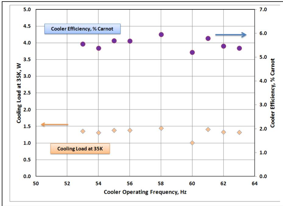
Figure 7 – Performance of 2 stage HEC cooler over a wide range of frequency
