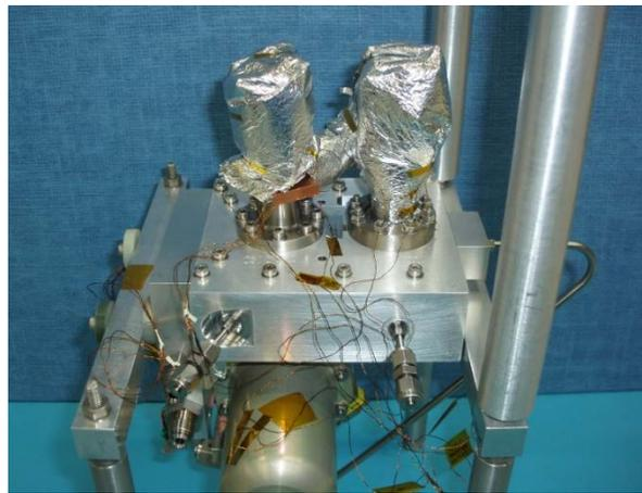
**Figure 4.** Integral configuration 2 stage coaxial cold head HEC in test fixture
