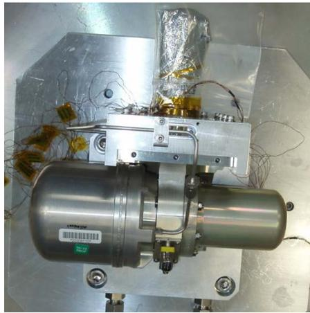
**Figure 1.** Single Stage HEC cooler with Coaxial Cold Head
