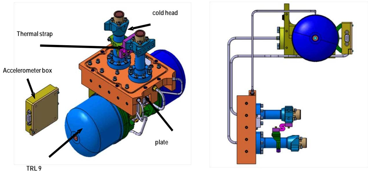
**Figure 5.** 2 Stage Cooler with Coaxial Cold Heads
