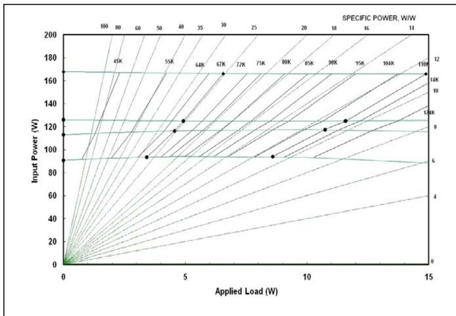
**Figure 2.** Coaxial HEC cooler performance map
