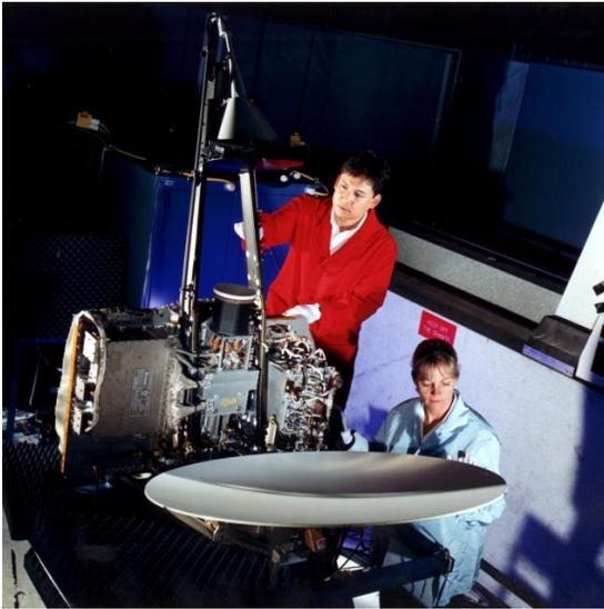
The LDR payload is built around a rectangular, box-like structure called the wing. Its major electronic subsystems are contained on four hinged panels which fold into this structure. The payload includes five major subsystems:
