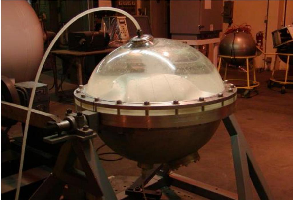
**Figure 3 Thruster Firing Tank**
