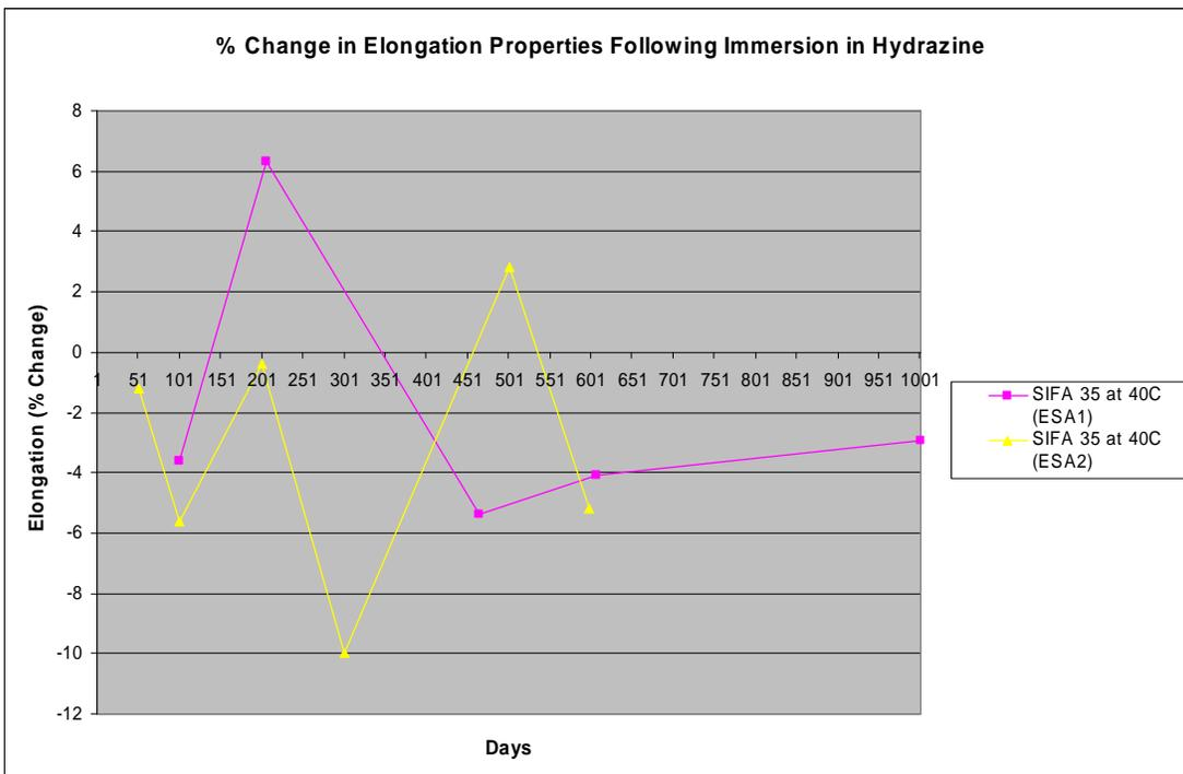
**Figure 6 % Change in Elongation Properties Following Hydrazine Immersion**
