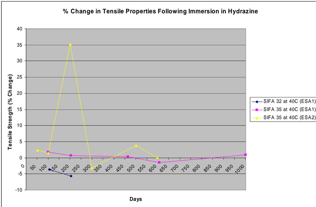
**Figure 5 % Change in Tensile Properties Following Hydrazine Immersion**
