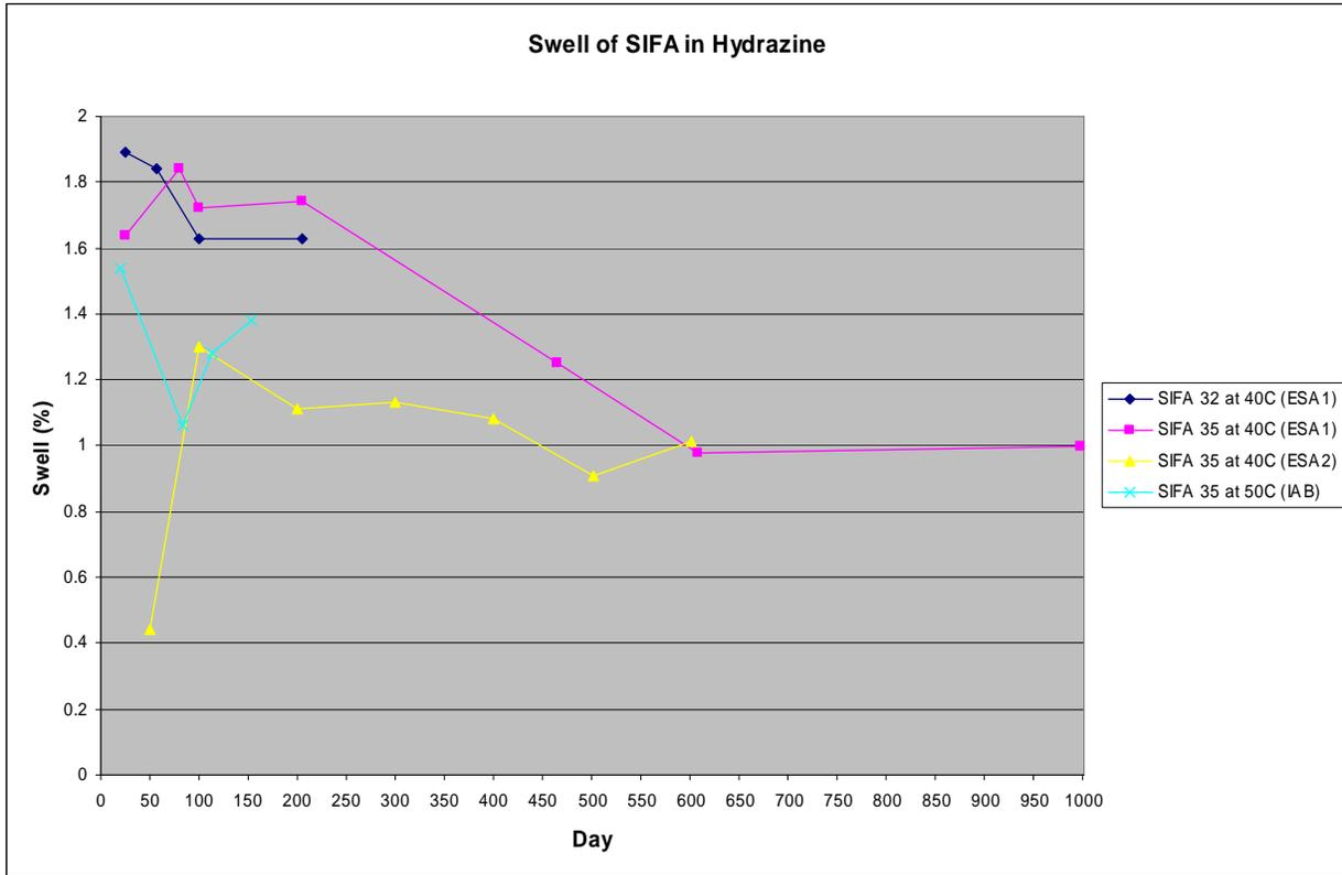
Figure 4 – Swell of SIFA in Hydrazine
