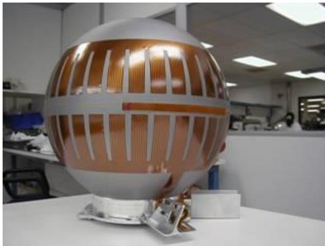
**Figure 5: Pressurant Tank Assembly shown with heaters, sensors, cables and flight bracket installed.**
