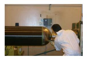
To complete the tank shell, a mounting plate is bonded to the tank cylinder section near the propellant end as shown in Figure 14.
