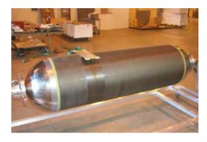
The oxidizer tank is stabilized with struts that are attached to flexplates on the upper pressurant port and the lower propellant port. The flexplates are added to the ports after final machine.
