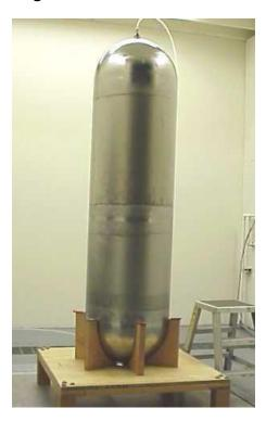
The welded liner is stress relieved in a vacuum furnace to reduce the stresses caused by the girth welds. Following stress relief, G40-800 fibers are applied over the tank cylinder section to complete the overwrap. See Figure 13.
