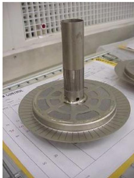
In addition, the PMD has been designed to prevent gas from penetrating the perforated sheet and exiting the tank during all applied loads. The flow path of the propellant is illustrated in Figure 7. The propellant flows into the sponge radially. The propellant within the sponge flows between and through the sponge panels into the perforated sheet preventing gas penetration.
