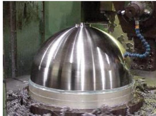
**Figure 11: A Machined Pressurant Head**
