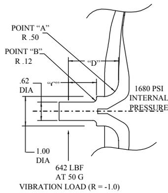
**FIGURE 10. STINGER END FITTING VIBRATION FATIGUE ANALYSIS @ 1680 PSI**
