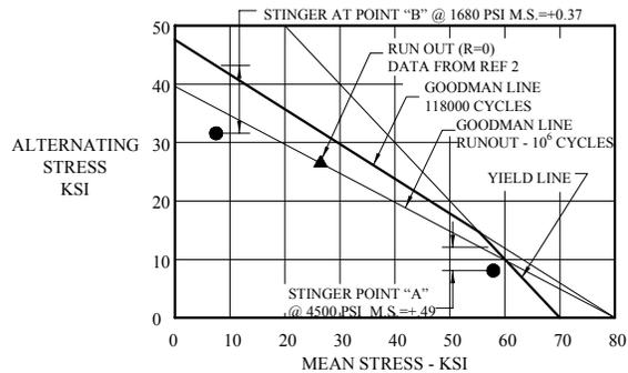
**FIGURE 4. ESTIMATED FINITE FATIGUE LIFE OF CP-70 TITANIUM**
