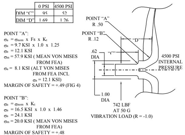
**FIGURE 9. STINGER END FITTING VIBRATION FATIGUE ANALYSIS @ 4500 PSI**
