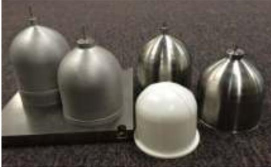
Figure 34:  $\varnothing 112$  mm ( $\varnothing 4.4$  in) Domes Made From Machined Domes and AM Domes
