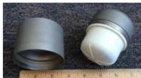
Figure 33: A Ø68 mm (Ø2.7 in) Tank Shell Made Using Additive Manufacturing Techniques
