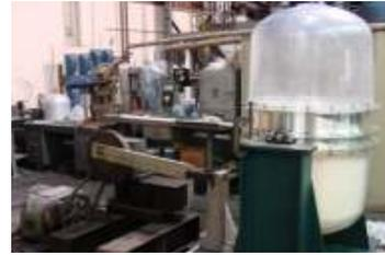
Figure 27: Slosh Test Setup
