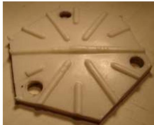
Figure 13c: Diaphragm Extrusion Test with Ribs Directly Above the Outlet and at 150 psig for 90 minutes
