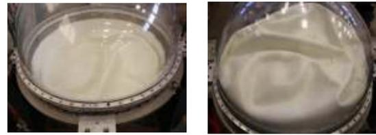
*Figure 16: Diaphragm Configuration at Lower Fill Fraction and High Fill Fraction*
