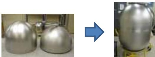
Figure 9a: A Diaphragm Tank Liner with Domes Having Cylinder Extensions and One Girth Weld
