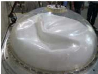
Figure 21b: *Improved Diaphragm Configuration with Folds but no Overlap at Higher Fill Fraction*
