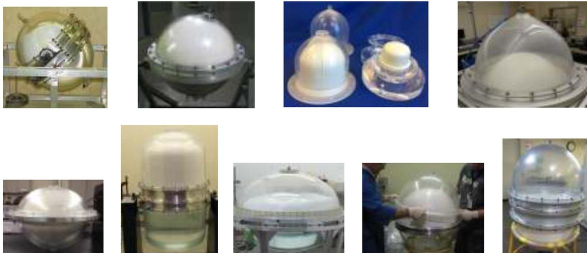
Figure 19: Diaphragm Tank Simulators of Various Sizes
