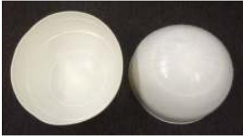
Figure 29: Adding Concentric Stiffening Rings to the diaphragm Interior Wall
