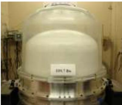
Figure 26: The Diaphragm in a Fully Reversed Position
