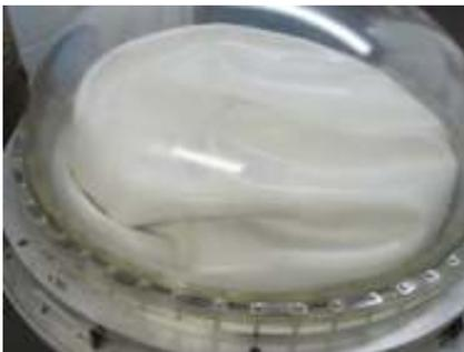
Figure 21a: *Folds and Overlaps Occurring at Low Fluid Fill Fraction*
