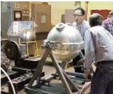
*Figure 15: A Slosh Test Setup to Examine Diaphragm Behavior in a Slosh Environment*
