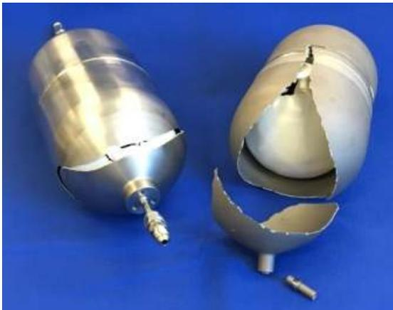
Figure 35:  $\varnothing 112$  mm ( $\varnothing 4.4$  in) Diaphragm Tanks after Burst Pressure Tests
