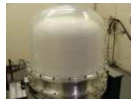
Figure 10b: An Example of a Fully Reversed Diaphragm Not Touching the Pressurant Dome
