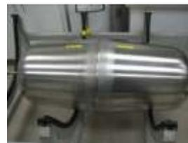
Figure 11: A Liner with Ellipsoidal Domes and Conical Bodies
