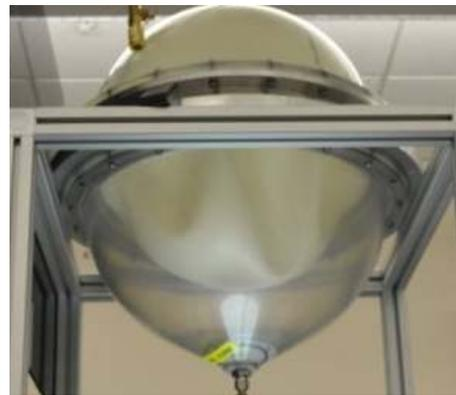
Figure 23: *Simulator for a  $\varnothing 419$  mm ( $\varnothing 16.5$  in) Diaphragm Tank Slosh Experiment*
