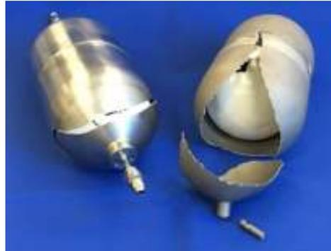
Figure 5: The two burst tanks. The additive manufactured tank shell is on the right.
