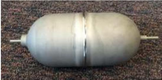
Figure 3: The welded QT2 tank with two additive manufactured domes
