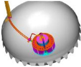
Figure 24: The PMD concept for P/N 80570 Hydrazine Tank
