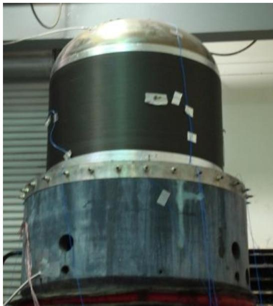
Figure 12: the P/N 80507 Qualification Tank during vibration testing
