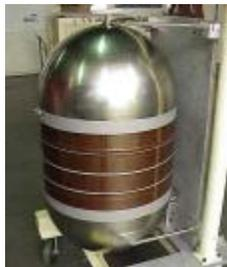
Figure 5: The MESSENGER shell manufacture took advantage of existing 22 inch diaphragm tank tooling
