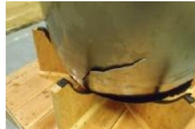
Figure 22: P/N 80520 Qualification Tank after Burst Pressure Test
