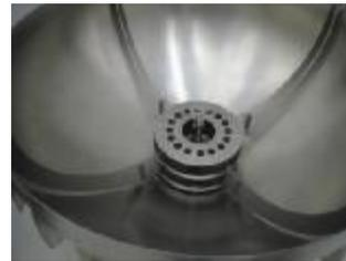
Figure 10: the P/N 80507 PMD installed in a finish machined tank shell
