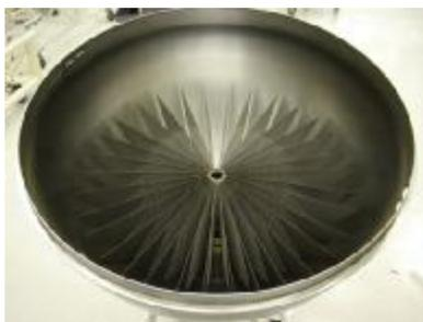
Figure 2: The SDO PMD installed in a modified PMD tank shell
