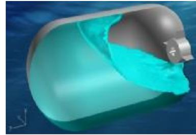
Figure 9: P/N 80507 tank horizontal handling analysis
