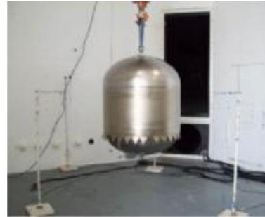
Figure 21: P/N 80520 Qualification Tank during Acoustic Test
