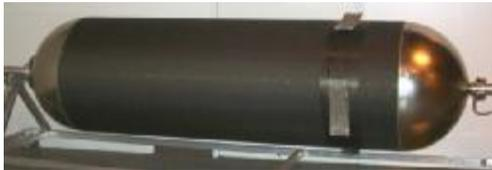
Figure 4: The Astrolink shell took advantage of existing 35 inch PMD tank tooling
