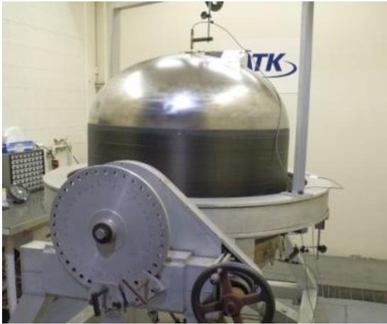
Figure 11: the P/N 80507 Qualification Tank during pressure testing
