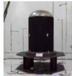
Figure 26: ATK P/N 80570 Qualification Tank Acoustic Testing
