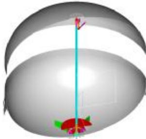
Figure 25: The PMD concept for P/N 80571 NTO Tank
