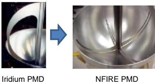
Figure 1: The Iridium PMD and the NFIRE PMD in the same shell
