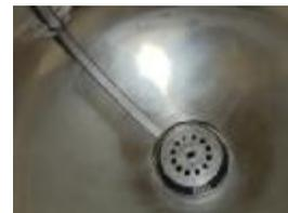
Figure 17: ATK P/N 80520-1 PMD as installed in the propellant dome
