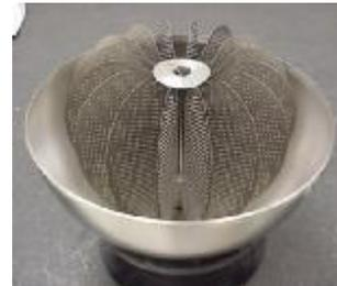
Figure 3: The Orbital Express PMD installed in a modified diaphragm tank shell
