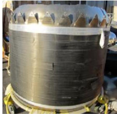
Figure 13: the P/N 80507 Qualification Tank after the destructive burst test
