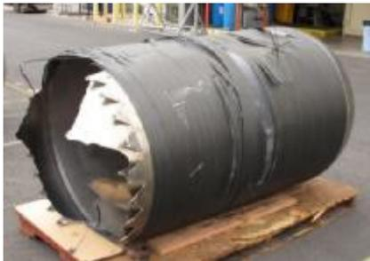
Figure 31: ATK P/N 80576 tank after burst
