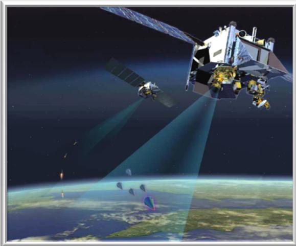
acquisition sensor that monitors and autonomously detects and tracks missiles during boost phase.
