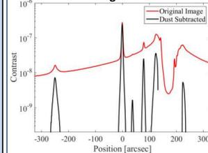
The mean of a 50 pixel slice through our best contrast image on a log scale with and without dust. For the dust subtracted case the background is approximately zero. The slice contains the edge of the 4km source, which is visible on the left
