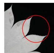
Sine wave introduced on top of the nominal petal shape. Frequencies: 25 and 50 cycles/petal length. Amplitudes: 0.1 and 0.15cm.
