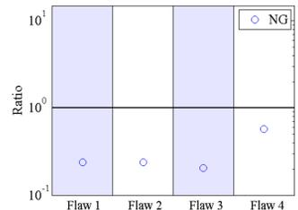
**Ratio Plots:** Above are plots that show the ratios of contrast flaw peak predictions generated by the numerical models (developed independently by Northrop Grumman, University of Colorado, and Jet Propulsion Laboratory) to the flaw peaks measured in the field. The black line represents the value measured in the field, and each point represents the ratio of the model prediction to that value. For the 2015 data set, JPL and CU models have not yet been run.
