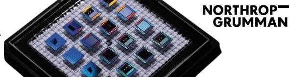
Preliminary Thermal Properties with die mounted with 25um 80/20 AuSn Eutectic to: 10mil Cu10W Shim.
