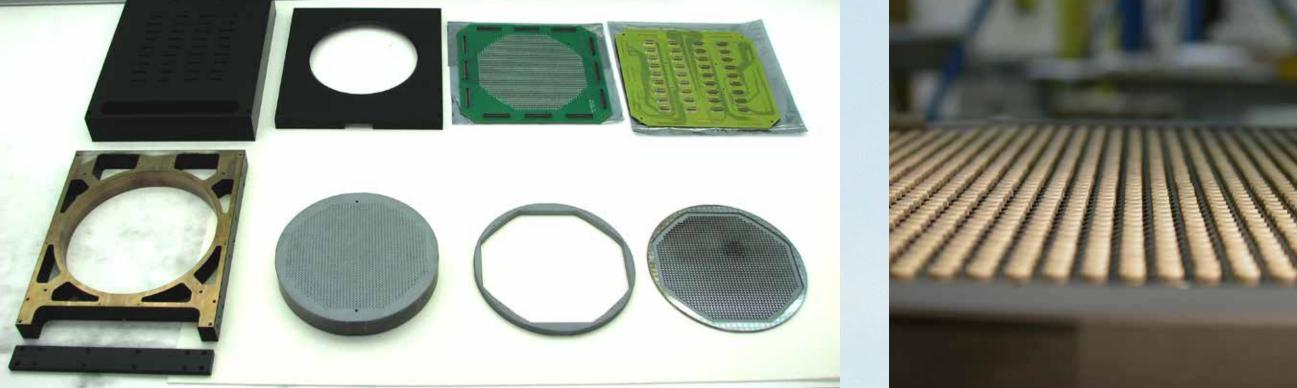
AOX, the leading supplier of precision DMs, produced the DKIST DM using our proven lead magnesium niobate electro-ceramic actuators. The DKIST AO system requirements resulted in a unique, thermally-controlled 1600 channel DM with an actuator pitch of 4.7 x 4.9 mm, 5 microns of available stroke and an interactuator stroke limit of 2 microns. At full solar illumination the thermal system controls facesheet temperature from +0 to -2 °C from ambient. AOX is proud to be a member of the DKIST team.
