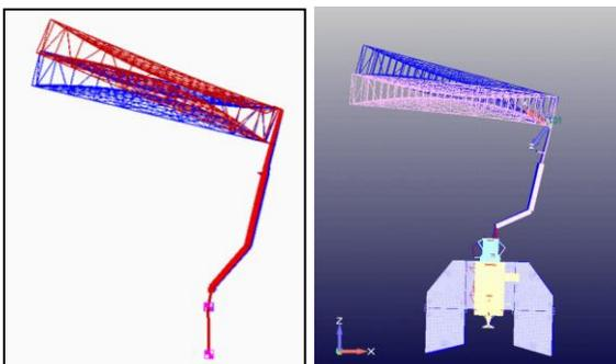
Figure 14. 1<sup>st</sup> Free-Free Structural Mode, 1.8 Hz
