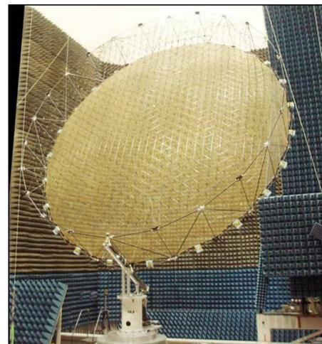
Figure 4. AM-Lite EQM 50GHz Performance Test at NASA GRC
