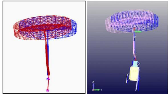
Figure 15. 2<sup>nd</sup> Free-Free Structural Mode, 2.3 Hz
