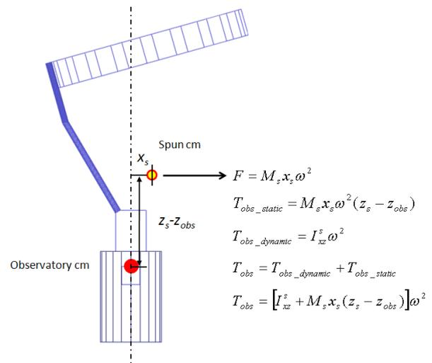
Figure 17. Observatory Balancing
