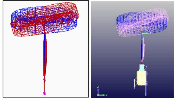
Figure 16. 3<sup>rd</sup> Free-Free Structural Mode, 3.3 Hz
