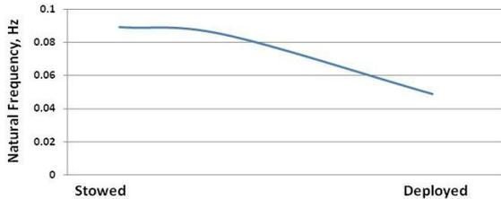
Figure 10. Natural Frequency - Boom Deployment
