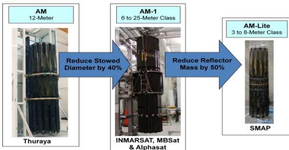
Figure 3. AstroMesh Reflector Family Evolution
