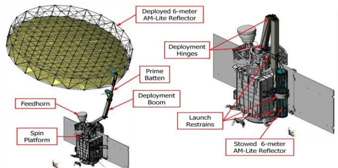
Figure 5. RBA Assembly on SMAP Spacecraft
