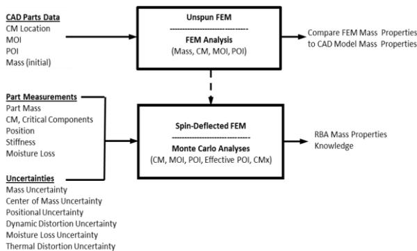
Figure 20. Flowchart for Mass Properties Analysis
