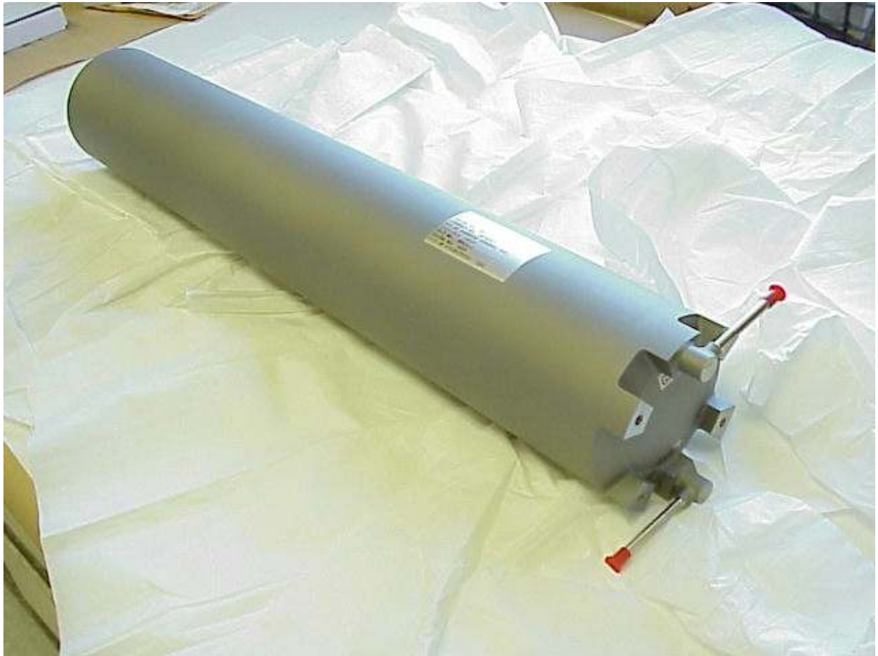
ORBCOMM Propellant Tank 80421-1
