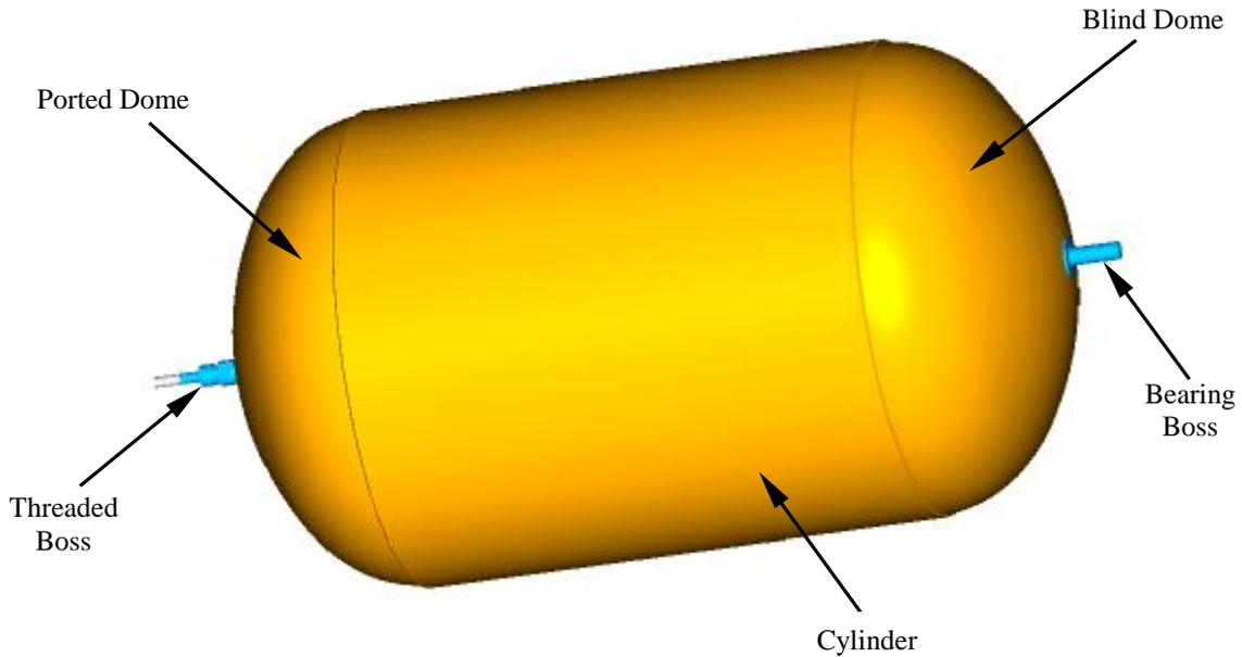
The tank is mounted to the spacecraft by polar bosses located on the tank centerline axis. The ported end is the fixed end with a threaded attachment to mount onto the spacecraft structure. The blind end stinger boss, mounted on a slip joint bearing, is designed to
