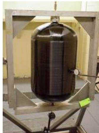
**External Leak Test:** The external leak test verifies the integrity of the tank shell and also serves to validate the previous series of pressure testing. The tank is placed in a vacuum chamber, which is evacuated to under 0.2 microns of mercury, and helium pressurized to MEOP for 30 minutes. The helium leak rate cannot exceed  $1 \times 10^{-6}$  std cc per second after a 30-minute stabilization period. For example, the leak rate of the Qualification Tank was  $2.3 \times 10^{-8}$  scc/sec.
