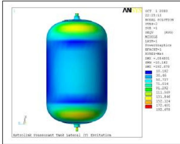
Figure 5b: Vibration Analysis, Axial Random Stress Response of Liner
