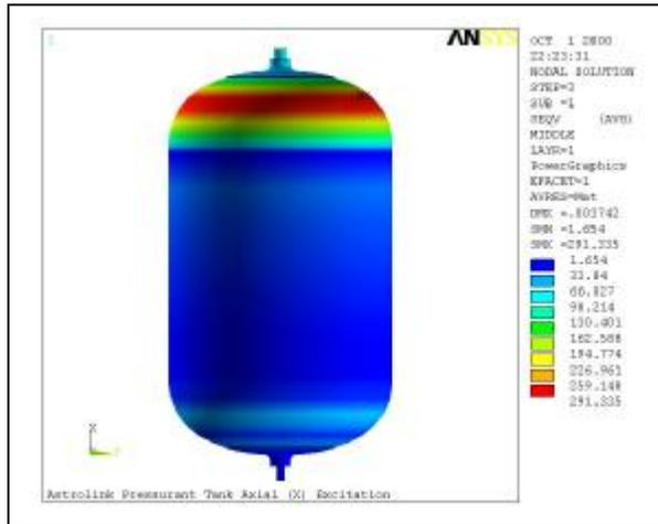
Figure 6: Liner Shock Response, Axial and lateral
