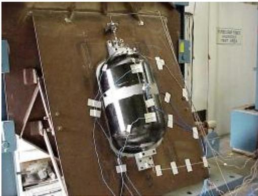
**Vibration Test, Sinusoidal and Random:**
