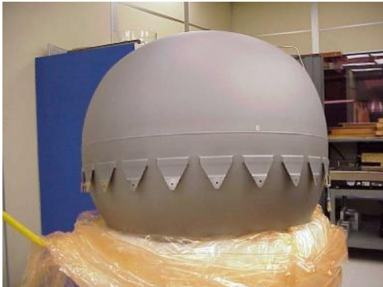
The all-titanium propellant management device is a combination radial sponge with integral propellant motion baffles, perforated sheet pickup assembly, and vanes.
