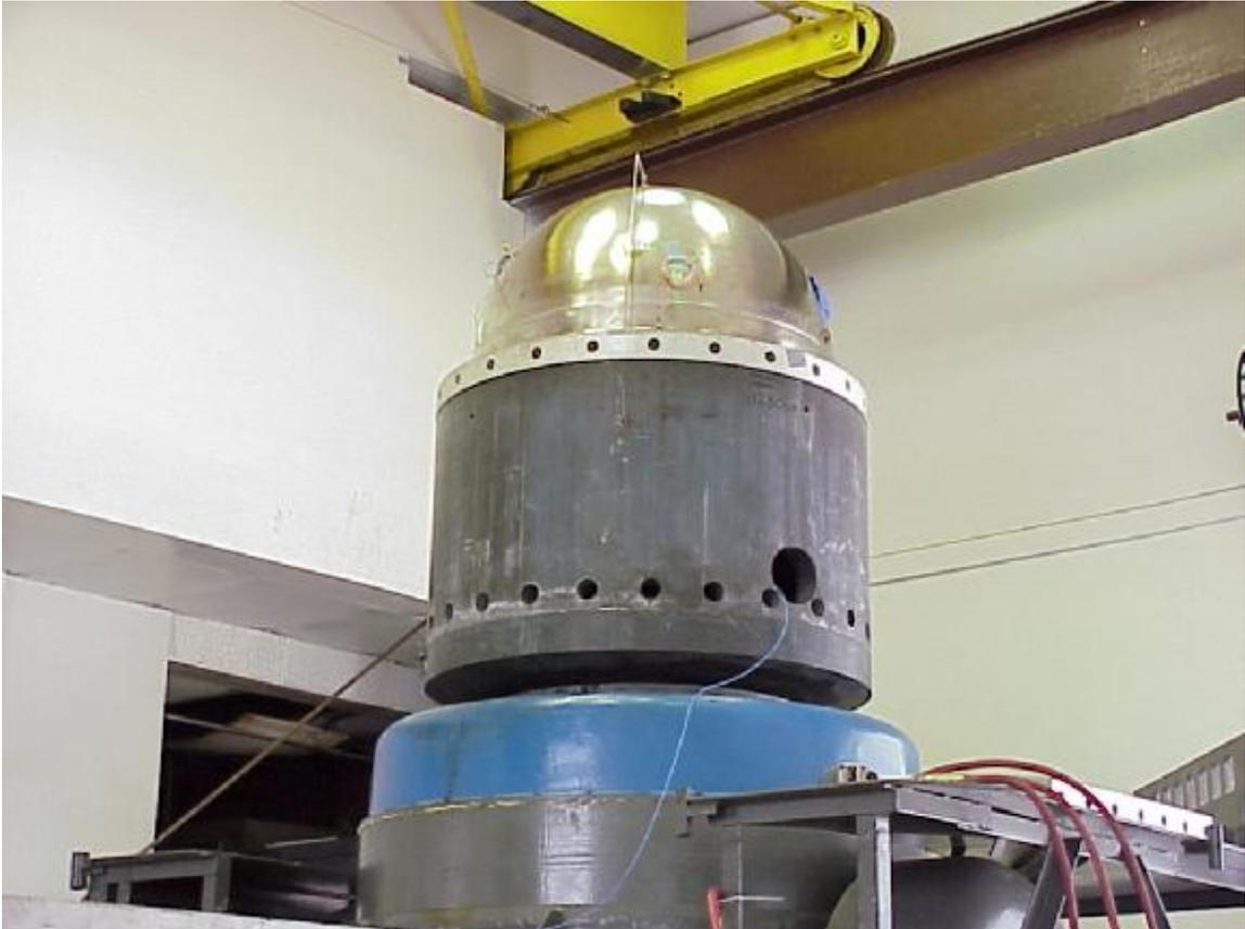
**FIGURE 14: PROPELLANT TANK IN THE PROOF PRESSURE TEST FIXTURE AT PSI**
