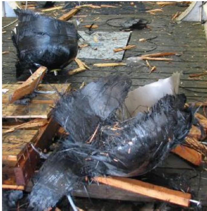
**Destructive Burst:** After the completion of the pressure cycles, thermal cycling and vibration testing, the Qualification Tank was subjected to a final destructive burst pressure test. The Qualification Tank burst at 904 bar (13117 psi), providing a 45% margin on burst pressure. This data represents a burst factor of 2.92 to 1, and a performance efficiency rating (PV/W) of 1.4. Figure 9 shows the Qualification Tank after burst.
