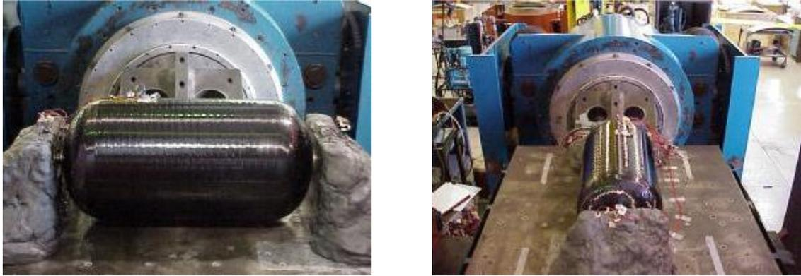
**Figure 9: Qualification Tank After Burst**
