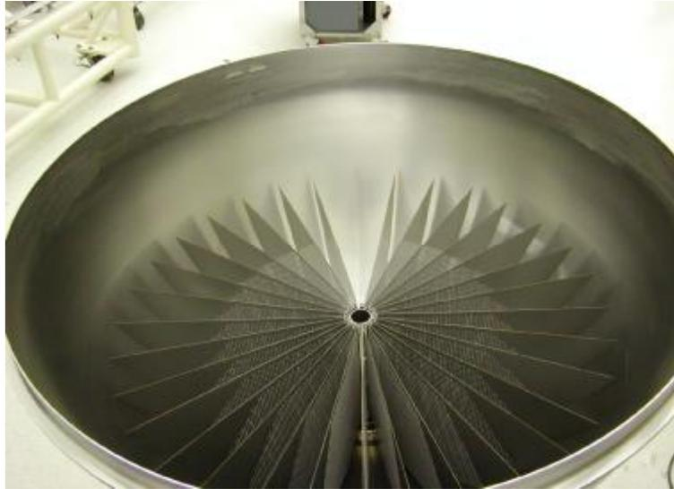
After PMD installation, the two heads are Tungsten Inert Gas (TIG) welded into a tank weldment. The completed tank assembly is shown in Figure 16.
