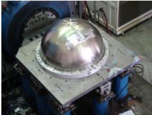
*Lateral Vibration Test Setup*
