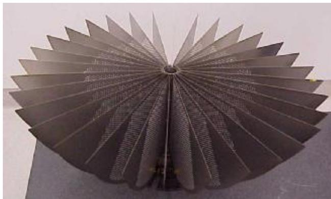
The PMD assembly is installed onto the propellant hemisphere assembly to complete the expulsion assembly, as shown in Figure 15.
