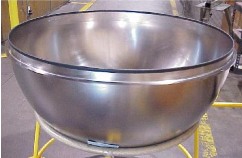
The PMD is manufactured separately in a parallel effort. The PMD components are fabricated from either titanium sheets or titanium bars, and welded into the PMD assembly as shown in Figure 14. This PMD assembly does not contain moving parts and, as noted earlier, is inherently reliable.
