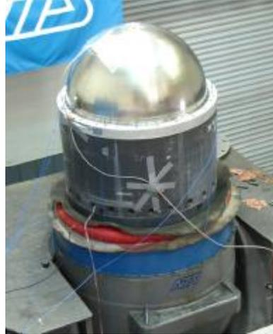
*Axial Vibration Test Setup*
