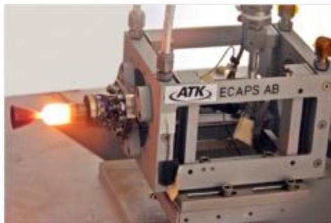
**Figure 2: 5 N HPGP Thruster (Courtesy ATK)**
