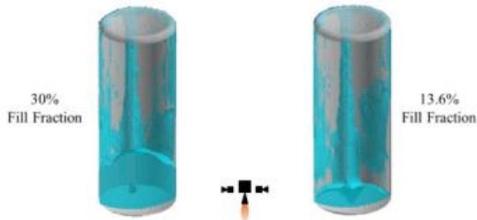
**Figure 9: Outputs of PMD functional analysis for 30% and 13.6% fill fractions: transient motion**
