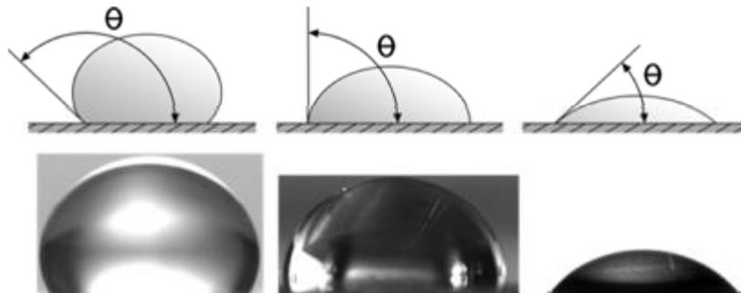
**Figure 5: Contact angles of various fluids, including LMP-103S, on various surfaces**
