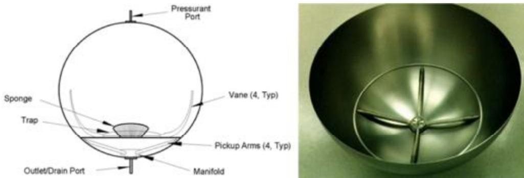
**Figure 1: Satellite propellant tank with propellant management devices [9] [10]**
