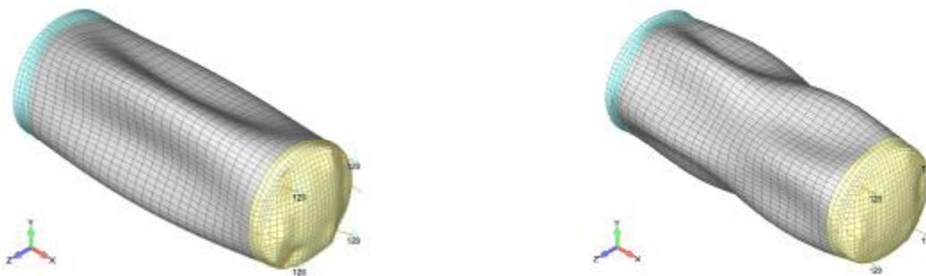
**Figure 7: Outputs of PMD tank structural analysis**
