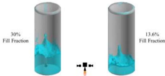
**Figure 10: Outputs of PMD functional analysis for 30% and 13.6% fill fractions: steady-state thruster firing**
