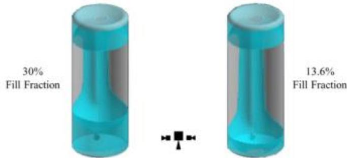
**Figure 8: Outputs of PMD functional analysis for 30% and 13.6% fill fractions: initial conditions**
