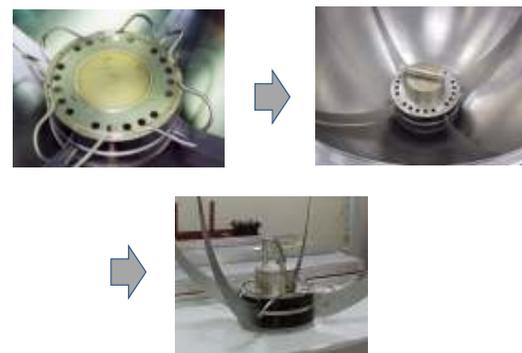
Figure 11, Evolution of PMDs to Accommodate Horizontal Handling
