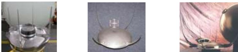
Figure 6c: Examples of PMD Assemblies with Multiple PMD Elements (Vaness, Sponges, Bulkheads for Traps)
