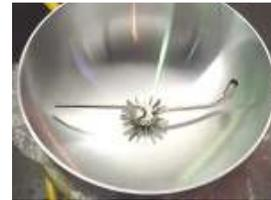
Figure 7: A PMD Mounted at the Tank Outlet Boss (one attachment point)
