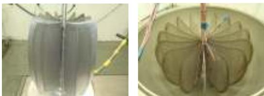
Figure 20, the JWST Hydrazine and NTO PMDs
