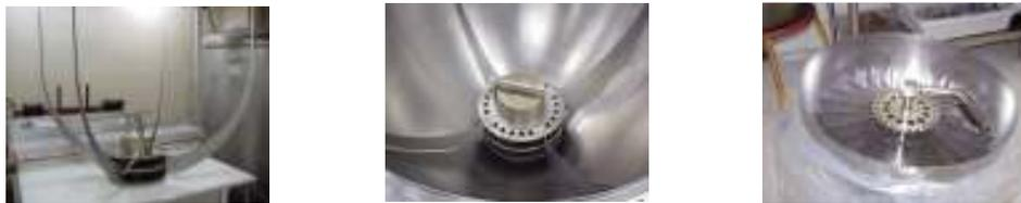
Figure 6b: Examples of PMD Assemblies with Multiple PMD Elements (Vaness, Sponges, Traps, Horizontal Handling Slosh Control Device)
