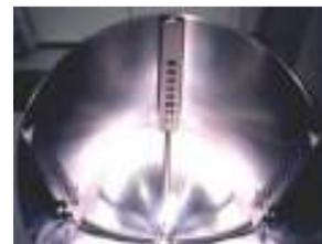
Figure 9: A PMD with Attachments on the Tank Shell (multiple attachment points)
