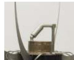
Figure 4c: A Horizontal Handling Slosh Control Device
