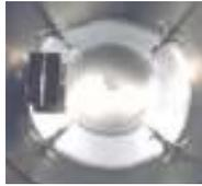
*Figure 10: A PMD Baffle Welded to the Tank Shell (attached circumferentially)*
