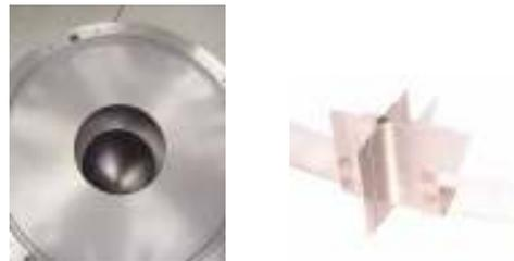
Figure 21, the MESSENGER Tank PMD
