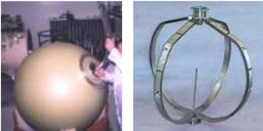
Figure 15, the Space Station ICM Tank PMD
