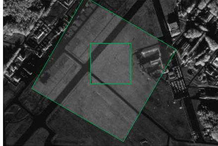
Northrop Grumman's advanced processing and proprietary algorithms automatically scan entire SAR maps, precisely locating and classifying targets of interest, and greatly reducing pilot workload.
