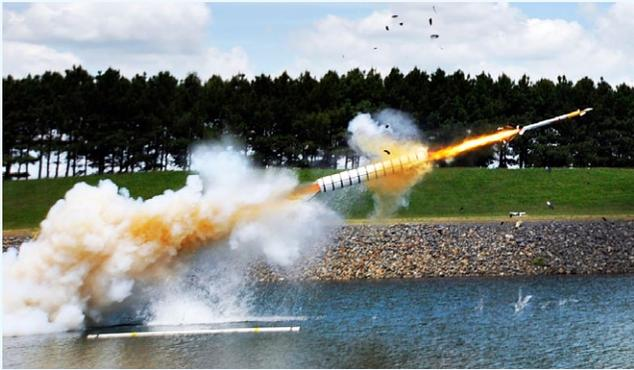
We adapted and designed the system used to launch Tomahawk cruise missiles, to help Raytheon Missile Systems successfully launch an AIM-9X air-to-air missile from underwater.
