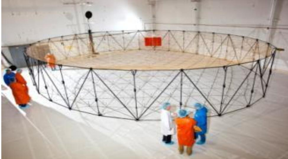
Figure 6. Verification testing of the Alphasat reflector at Northrop Grumman Astro Aerospace's cleanroom facility in Carpinteria, CA.
