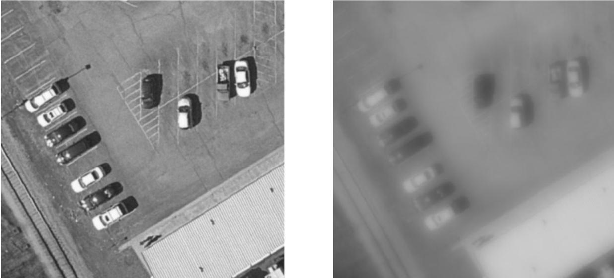
Figure 10. Raw image data from a fully filled pupil (left), and a thin, annular pupil (right), prior to post-processing.
