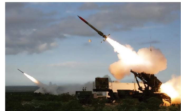
Patriot Advanced Capability 3 (PAC-3) surface-to-air missile being fired from its launcher. The missile is capable of intercepting not only cruise missiles but also UAVs and ballistic missiles. (Photo credit: U.S. Army)
