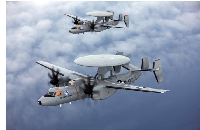
Northrop Grumman's AEW&C aircraft E-2D "Advanced Hawkeye." The U.S. Navy and the Japan Air Self Defense Force (JASDF) operate the aircraft. Its airborne radar covers hundreds of kilometers around. (Photo credit: U.S. Navy)
