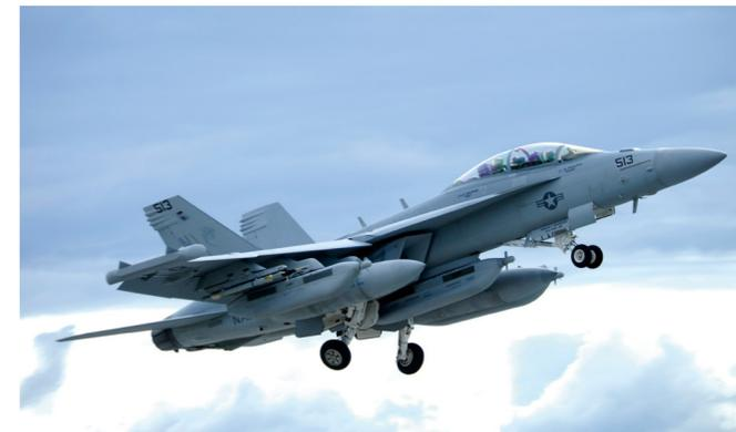
U.S. Navy's EA-18G Growler. The aircraft conducts various electronic attacks with the EW pods attached beneath the fuselage and at the wingtips. (Photo Credit: U.S. Navy)
