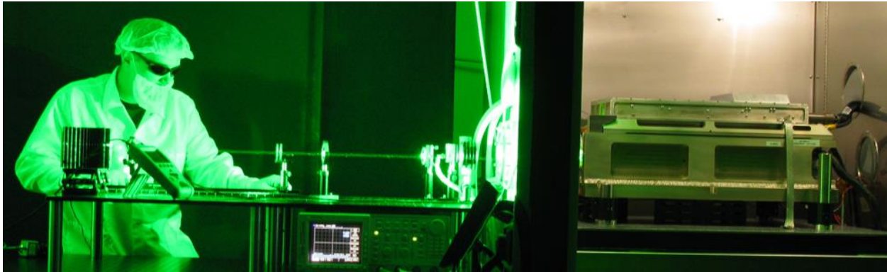
Figure 11: Laser in thermal chamber (right) undergoing operational thermal test (left).
