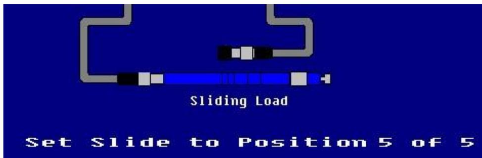
For slides with greater than the six position depicted, select the detents that will create a similar “two short and three long” pattern paying attention that all of the selected increment sizes are unequal in spacing.
